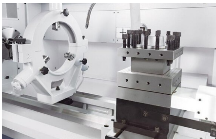
Heavy, automatic 4-station servo-driven tool changer for programmed tool changes
