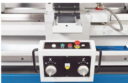
Compact control unit with electronic hand-wheels
